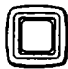
SECONDARY AIR TANK PRESSURE GAGE - Indicates tank pressure in psi and kPa
