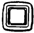
PRIMARY PRESSURE ALARM LAMP - Audiovisual signal indicates when pressure drops below 60 psi (410 kPa)
