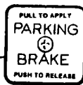
PARKING BRAKE CONTROL - Pull knob to apply parking brakes - Push knob to release brakes
