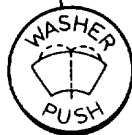
WINDSHIELD WASHER CONTROL - LEFT/RIGHT - Push knob to energize washer pump The pump stops when the knob is released
