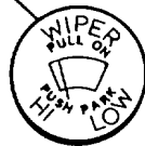
WINDSHIELD WASHER CONTROL - LEFT/RIGHT - Push knob to energize washer pump The pump stops when the knob is released
