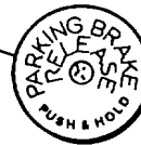
EMERGENCY PARKING BRAKE RELEASE - Push and hold control knob depressed to release parking brakes
